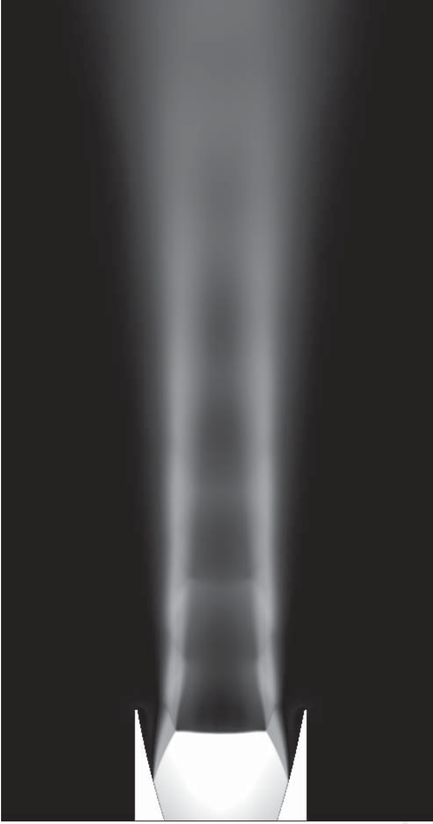
Average Mach number in a Detached Eddy Simulation (DES).
